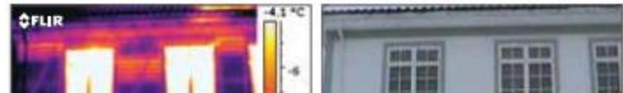
*Framework construction. Many of the sections are visible by the warmer colors.*
